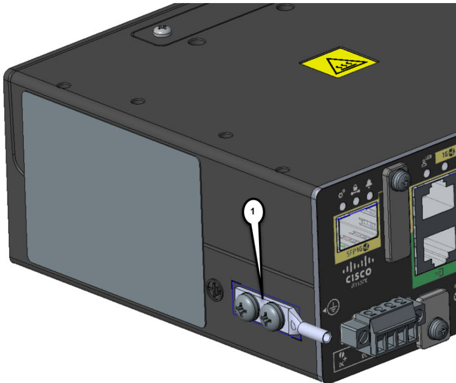
Figure 20: Chassis Ground Connection Points
